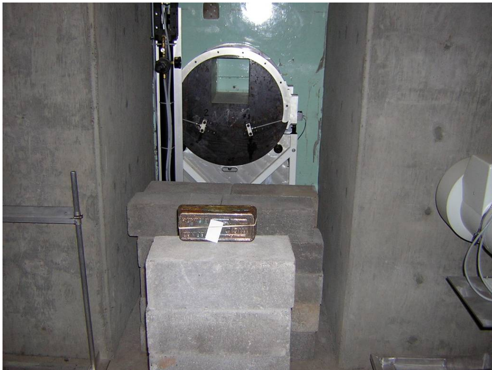
Figure 2. The shutter of the neutron radiography facility, the bismuth brick, and the concrete sample stand where sensing strips were held or irradiation.
