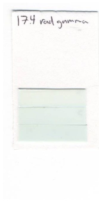
Figure 5. An example of sensing strips mounted on a paper card.
