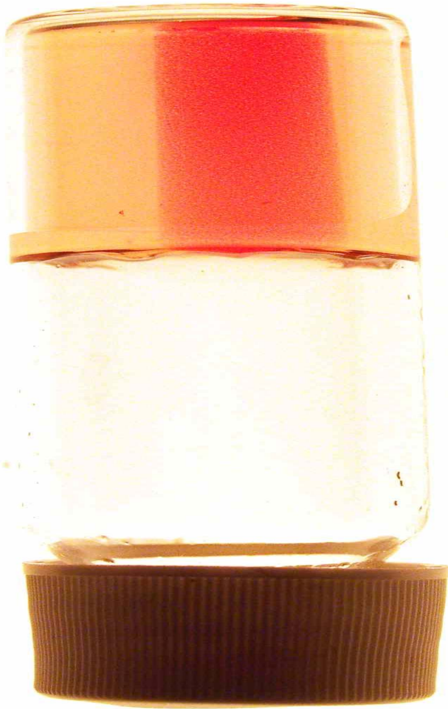
A side photograph of a plastic block in a vial irradiated with a narrow beam of 100 KeV X-ray
