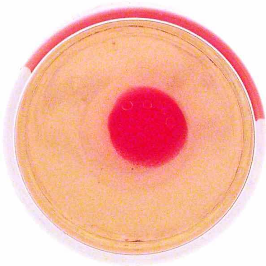
A top photograph of a plastic block in a vial irradiated with a narrow beam of 100 KeV X-ray
