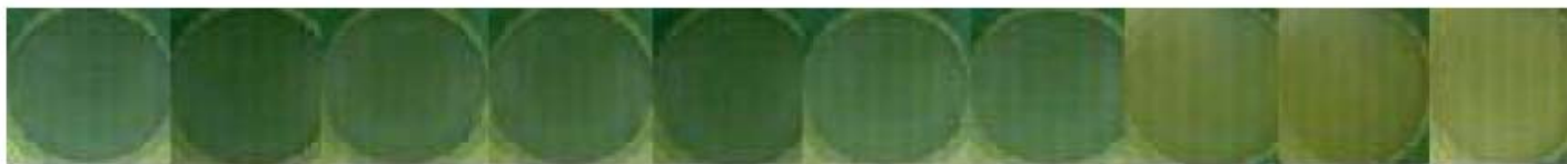
Figure 4-2. Color response of the Vitsab C2-10 TTI from activation to endpoint.
