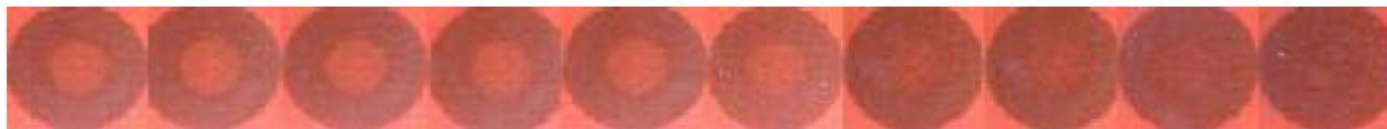
Figure 4-3. Color response of the Lifelines Fresh-Check TTI from activation to endpoint.
