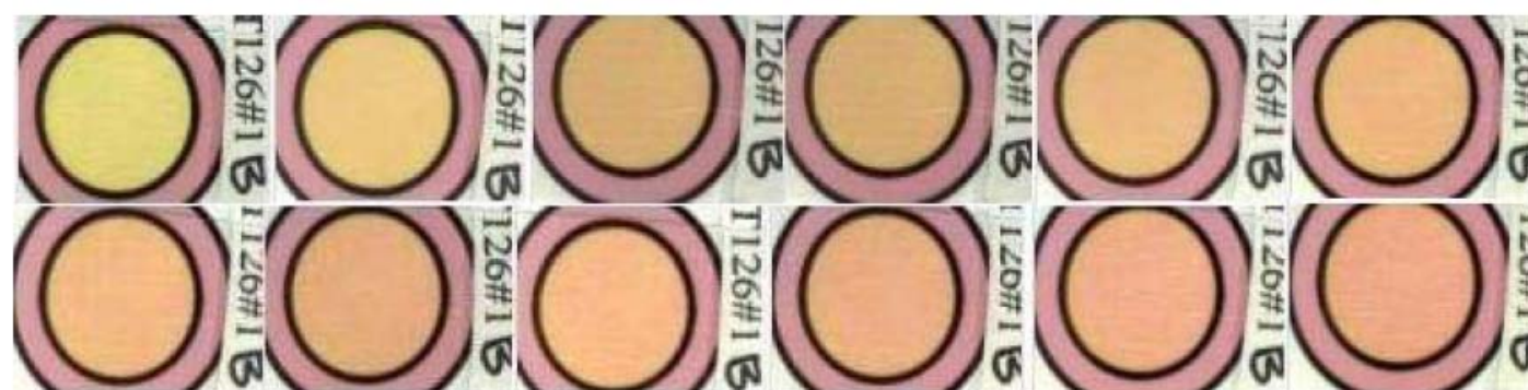
Figure 4-7. Color response of the Avery Denison T126(1) at 5°C over 12 days.
